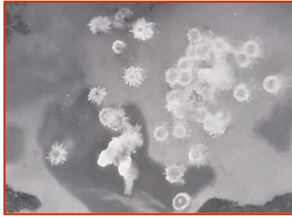
Bomb Splash Patterns - exhibit a concentric ring or radial pattern at impact.
