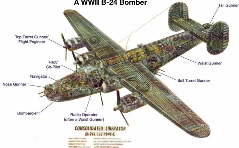
Drawing of a B-24 with crew positions
